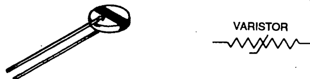
Figure 8-4 — A Silicone Carbide Varistor
